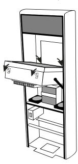
Step 5 Using caution not to twist the frame, lift off the face using the aluminum frame (may be tight) and leaving the ground strap in place, flip over the face so the holes in the frame can hang on the stainless steel face retainers.
