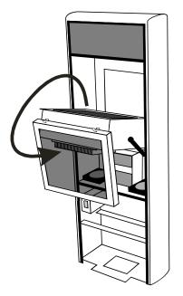
Step 6 Lift out the electronics insert and remove the old compact flash. Insert the new compact flash into the slot on the computer.
